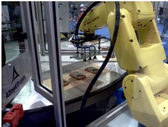
LR Mate 200iC Robot Loading Lip Gloss in an Aergo 8 (Left) and 4-Up EOAT for Loading Dental Floss (Right)
