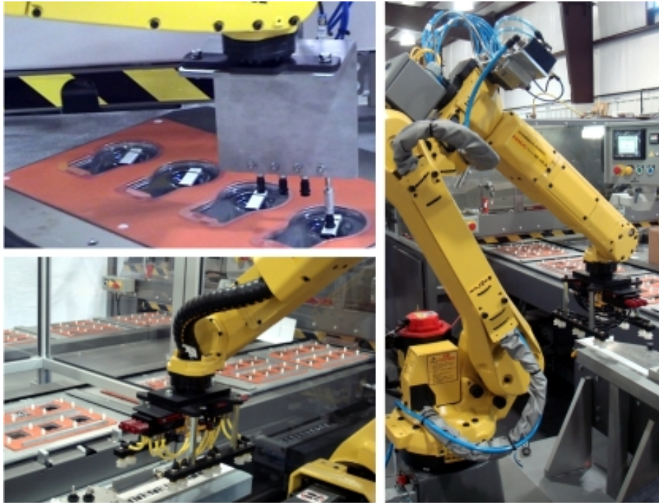
Loading USB Drives in an Aergo 8 (Top Left) and Batteries in an Aergo SL (Bottom Left and Right)
