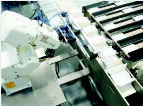
LR Mate 200iB Collating and Loading Blisters of a Drug Delivery Device into the Infeed of an Automatic Horizontal Cartoner
