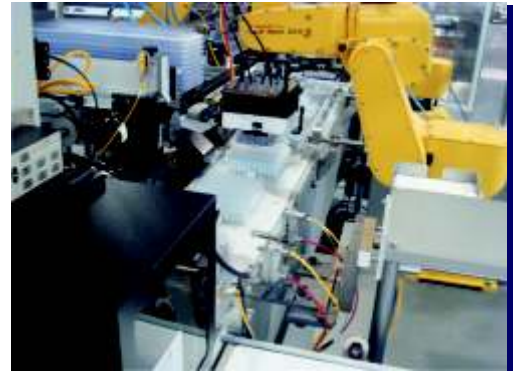
LR Mate 200iB Placing Tray Covers in a Pharmaceutical Tray Loading Application
