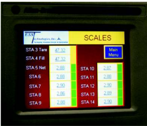
Tare and Gross Weights Are Recorded by the HMI
