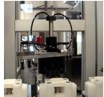
Cassette Halves are Joined to Complete the Test Kit Assembly
