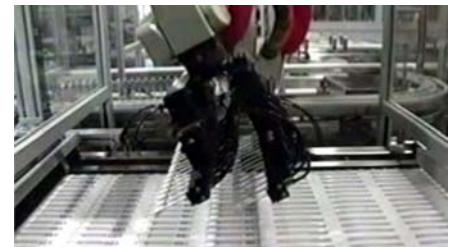
Robotic Loading of Thermoformed Blisters
