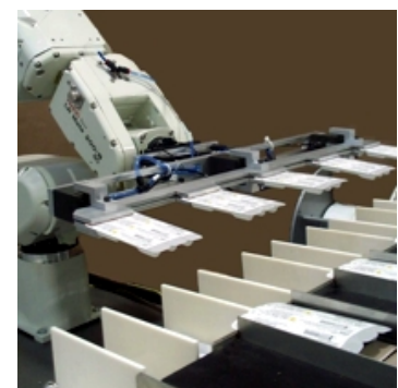
Collating and Loading Blister Packs into a Cartoner Infeed Bucket
