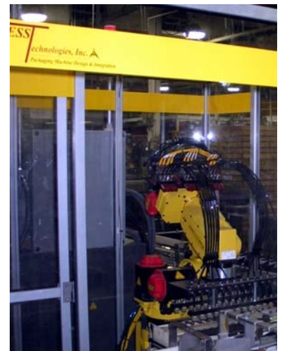
Robotic Cell for Loading Trays with Batteries
