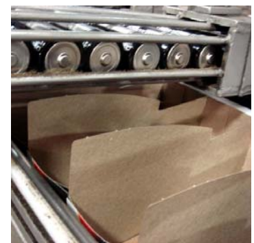
Batteries and Trays at Infeed
