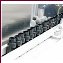
Infeeds designed for exceptional handling of vials, bottles, micro-tubes, etc.
