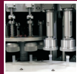
Servo pre-torque and final torque capping stations allow precise torque to be applied.
