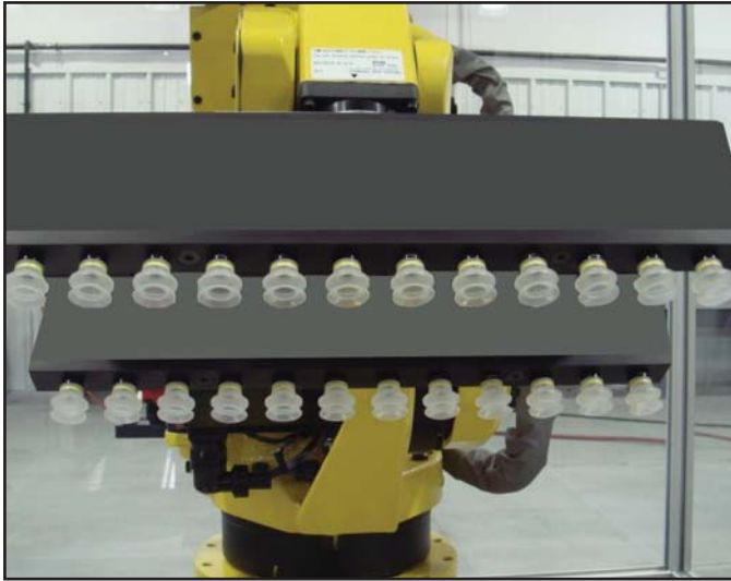
End-of-arm tooling for tray loading
