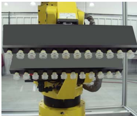
Custom Robot End-of-Arm-Tooling for a Loading D-Cell Batteries Into Blisters on a Blister Packaging Machine
