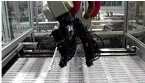
Robotic Loading of a Drug Delivery Device Into Blisters in a Thermoformer Machine
