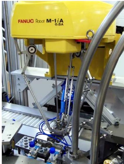
FANUC M-1iA Robot Unloading Vials from a Monoblock Filler/Capper and Placing Them on a Labeler Infeed Conveyor
