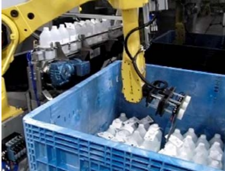
FANUC M-16iB Robot With Multi-purpose EOAT Nudges Pharmaceutical Bottles Into Place After Loading Them In the Crate
