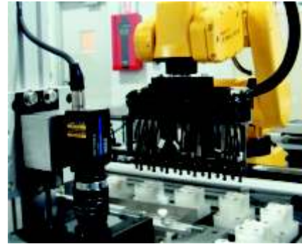
Vision Inspection Camera for Diagnostic Test Kits
