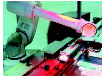
Robotic Infeed for Diagnostic Test Kit to Pouching Machine
