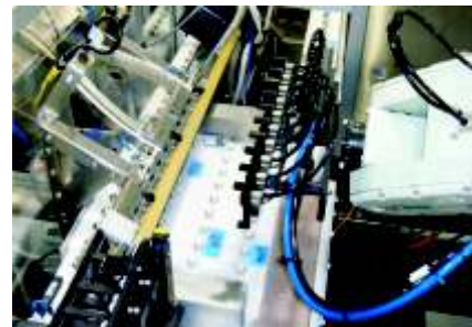
End Effector for Robotic Assembly of Drug Delivery Device
