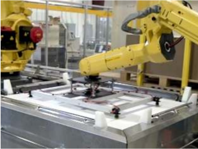
Top Cap Blank Placed On Former By Robot
