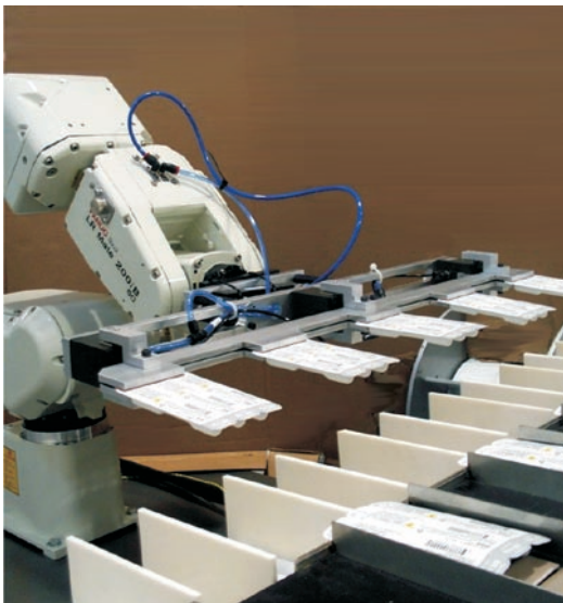
FANUC LR Mate 200iC Collating Blister Packs at a Cartoner Infeed
