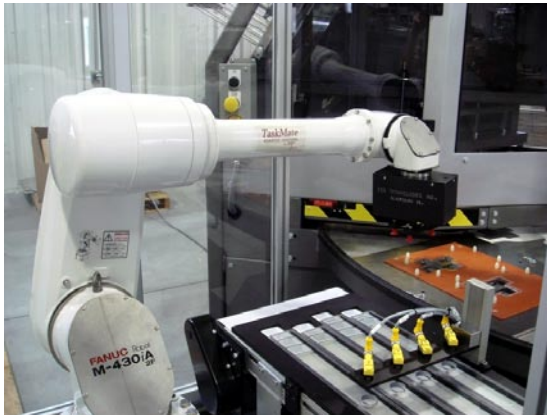
FANUC M-430iA Robot Loading Product Into Blisters at the Infeed of a Thermoform Blister Packing Machine
