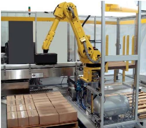
Dual Robotic Mini Palletizer Cell In A One-In, Two-Out Configuration
