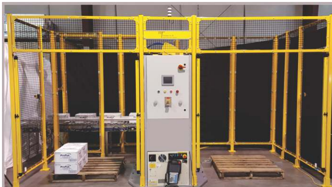
Dual Cell-E Configuration with Light Curtain Option
