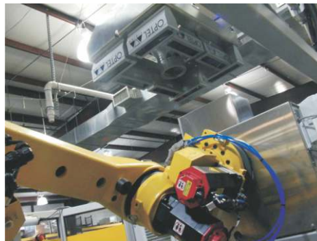
Integrated Overhead Vision System Verifies Case Load
