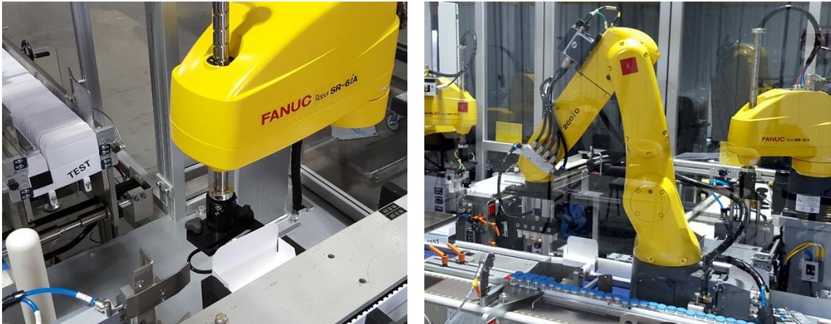
*SR-6iA Carton Erecting Robot and Robots for Partition, Vial and Leaflet Loading*
